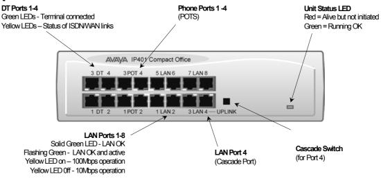
Note: The IP Compact Office DT4 is shown above. The IP Compact Office DT2 does not have the top row (labeled **3 DT 4**, **3 POT 4**, **5 LAN 6** and **7 LAN 8**) of RJ45 ports fitted.
